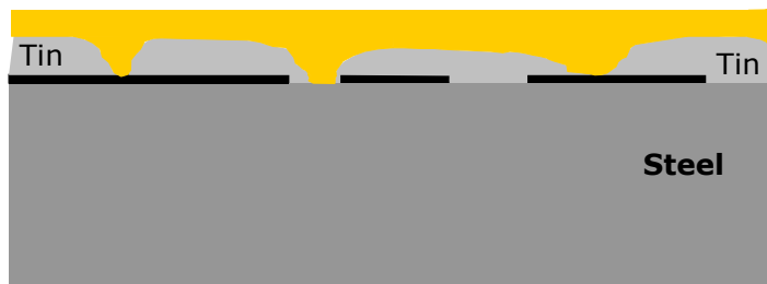
A polymer coating fills pores in a tin layer (coating)
