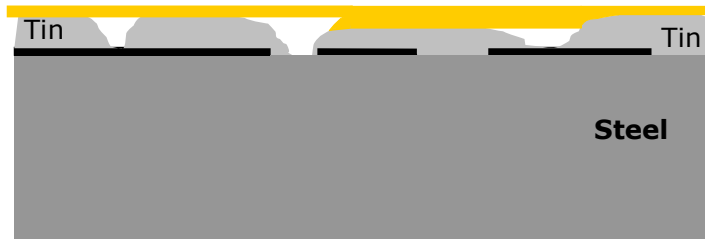
A polymer coating bridges pores in a tin layer (coating)
